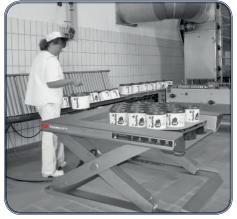
The stainless steel solution makes it perfect for rugged conditions and the use of aggressive cleaning products like in the food industry.
